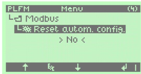
**Remark** To restart the detection the entry Yes has to be selected. If the reset was recognized by the control logic the display will return to No.
