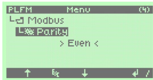
Remark This parameter will be ignored if the loop redundant version is selected and the automatic configuration is enabled.
