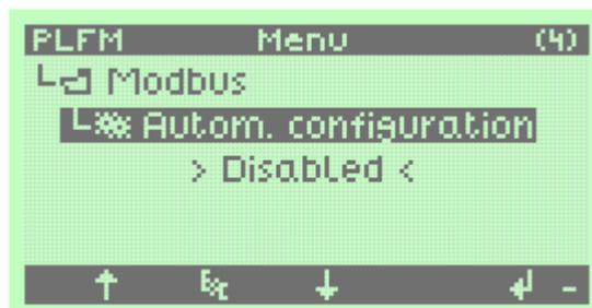
Remark The automatic configuration will only work with the loop redundant version if the interface. With all other versions this item will be ignored. If the automatic configuration is enabled the following parameters are obsolete:
