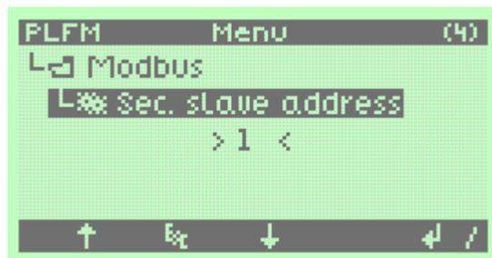
Remark The value 247 is reserved for new devices and should not be used in a real installation. The secondary address is only used with the master/slave version of the interface.
