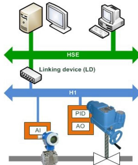
Figure 1: typical Foundation Fieldbus structure
