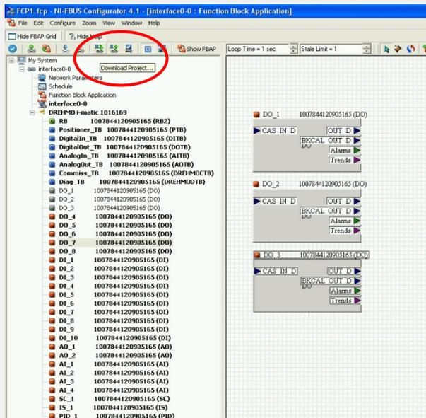
Figure 14: Download the function block application
