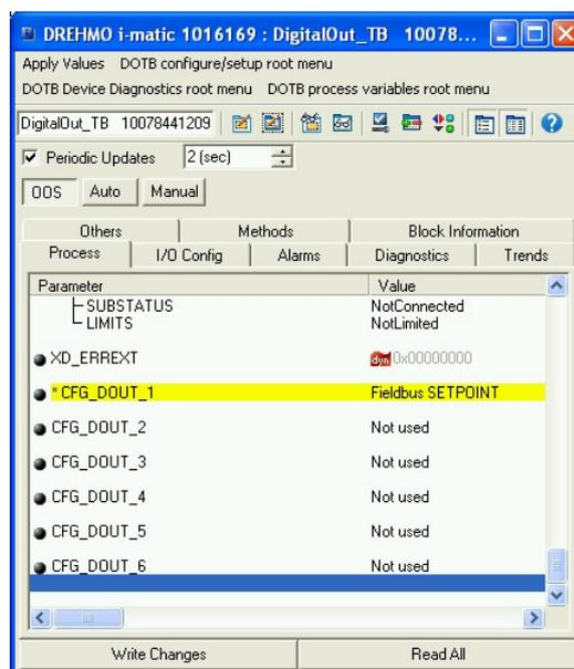
Figure 48: Assignment of the config. output from DOTB
