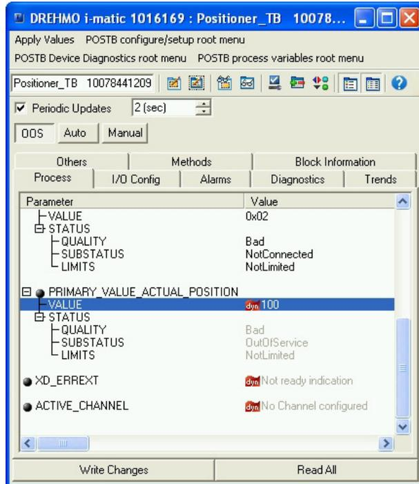
**Figure 54: Actual position value of the actuator**
