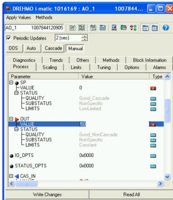
Figure 53: analogue control of the position setpoint
