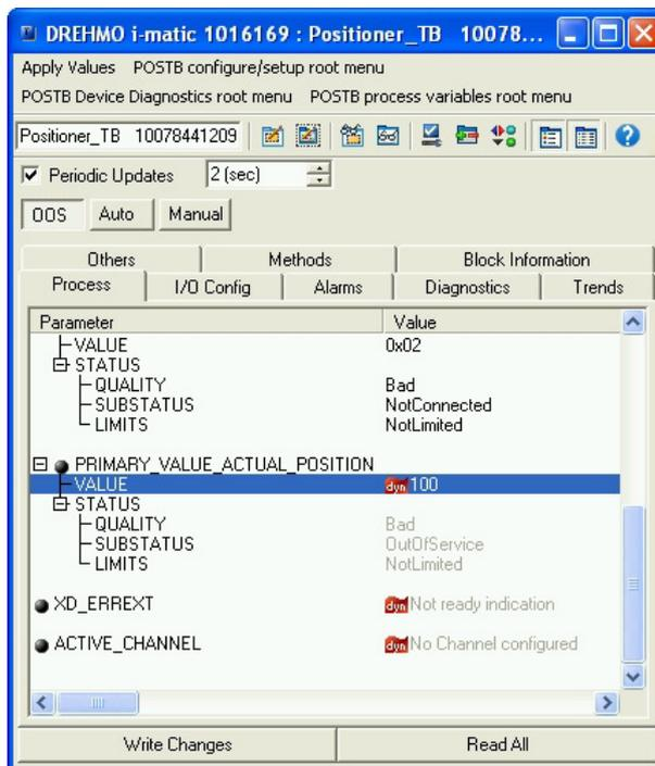
**Figure 22: Actual position value of the actuator**
