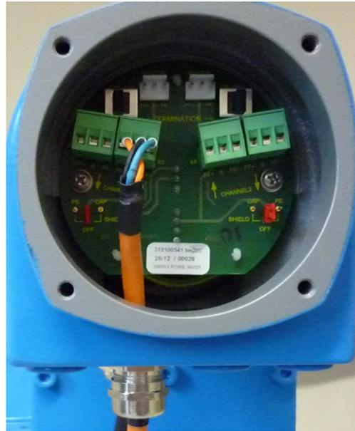
Figure 7: Bus connection board
