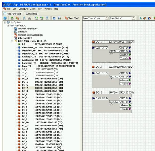
Figure 17: Representation of three DO function blocks
