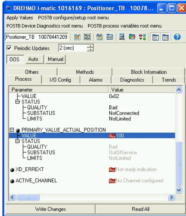
**Figure 44: Actual position value of the actuator**
