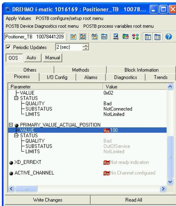
Figure 28: Actual position value of the actuator
