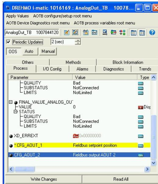
Figure 37: Assignment of the config. output from AOTB
