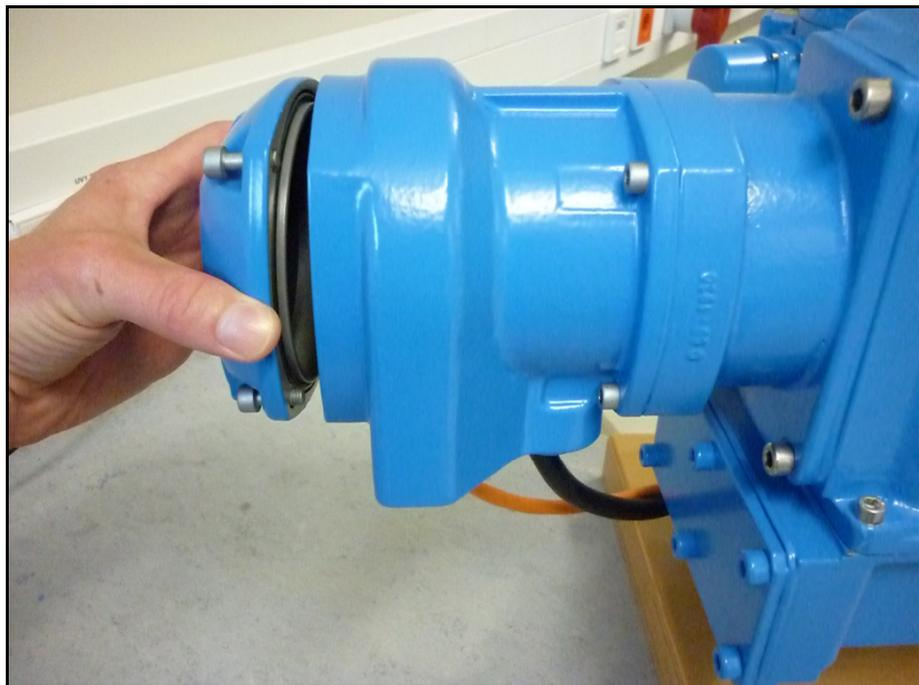
**Figure 9: Terminal compartment for Foundation Fieldbus**
