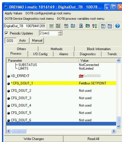
Figure 38: Assignment of the config. output from DOTB
