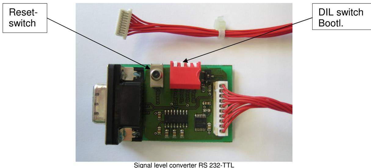
Signal level converter RS 232-TTL
