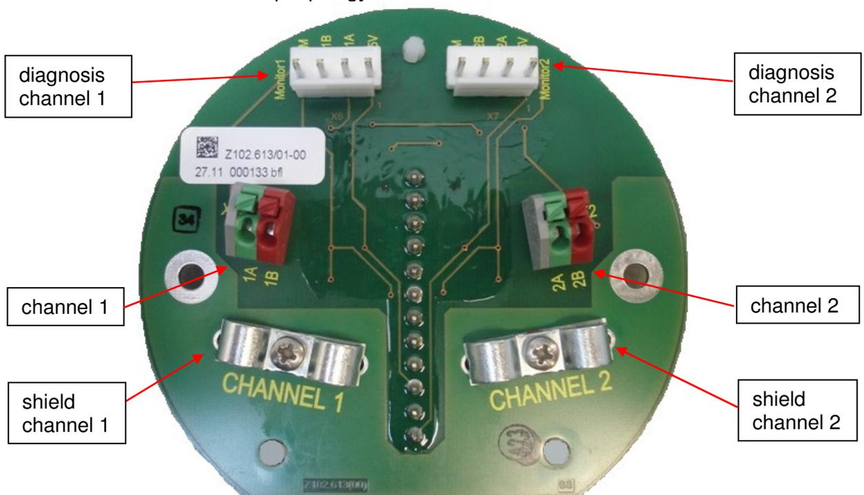
Connection board for modbus star / line topology (2 channel version shown):
