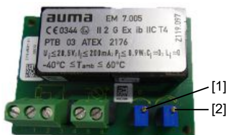
Figure 23: Electronic position transmitter B3 (EM7.005) in explosion-proof version
