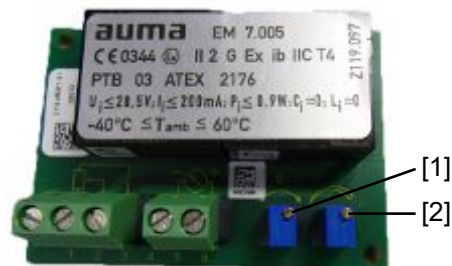
Figure 23: Electronic position transmitter B3 (EM7.005) in explosion-proof version
