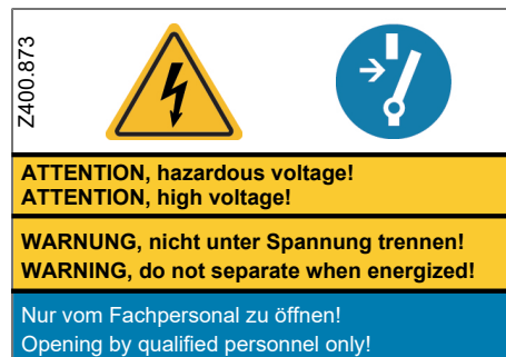
Figure 22: Label with warning of hazardous voltage
