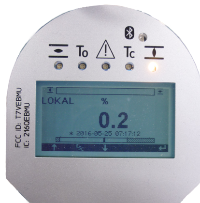
Figure 16: Display and indication elements of the local controls
