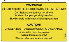
Exclude any kind of charge-generating processes (e.g. only wipe with a damp cloth, not with leather), as they can lead to ignitable electrostatic discharges. High charge generating processes are processes stronger than manual friction, e.g.:
