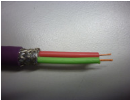
Preparation of the PROFIBUS cable and wires
