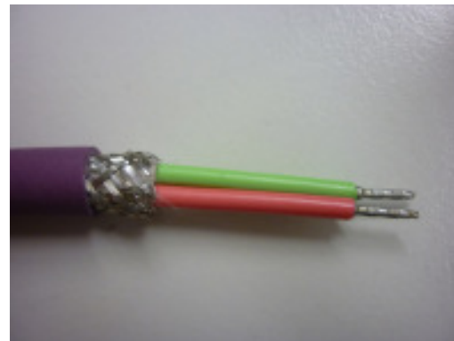
Preparation of the PROFIBUS cable and wires
